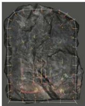
Figure 7: view of as planned (green point) and as drilled (red point) with a semi-automatic drilling machine
