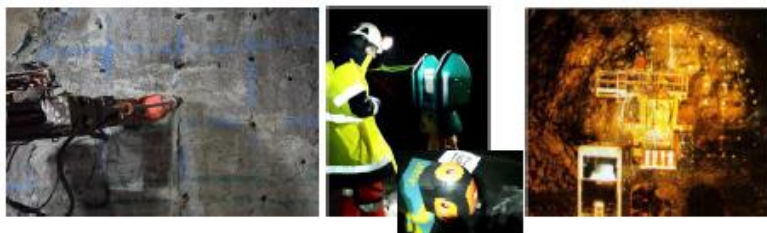
Figure 5: grid paint off face (left) — laser system projecting hole mark according to drilling pattern (center) — drill plan projected directly on the face with a digital projector (right)
