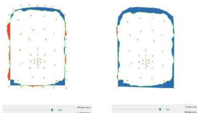
Figure 15: over break and under break measurement as planned vs drilled
