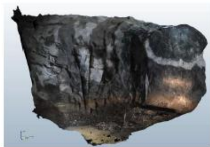
Figure 12: 3D model computed from pictures get with a classic camera (smartphone)
